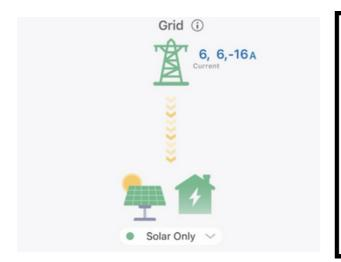
Solar Only mode will not work when all three (3) phases are exporting less than 20 Amps.
