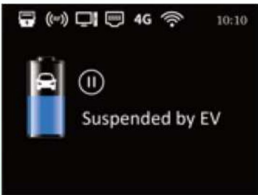
Suspended by EV - Indicator that charging session has been stopped by your EV e.g., limit set on car
