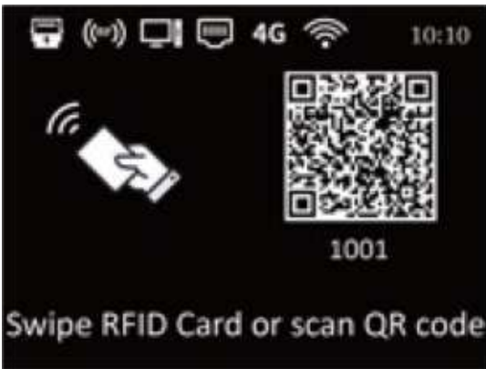
Scan the QR code or swipe the RFID card to start charging
