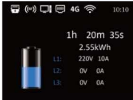
Charging in process - Shows Session Duration, Total power used, charging current and voltage per phase
