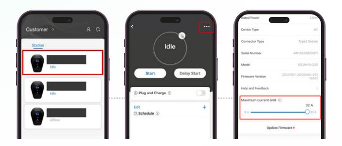
If the charger is still charging slow after changing both the Smart Charging Speed and Maximum Current Limit, check if the charger is set to Solar Only or Solar Assist mode following instructions from Section 3.
