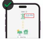
Solar Only mode will not work when all three (3) phases are exporting less than 20 Amps. This means that there is no clear excess when summing all three (3) phases.
