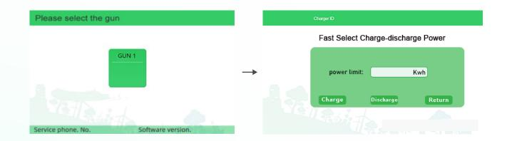
2. After choosing the charging connector/ charging power, click the confirmation button to initiate the EV charging process, as shown below.
