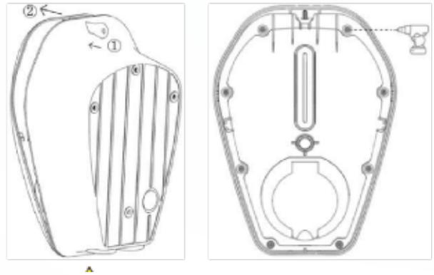
3. Unclip the communication cable and put the front panel aside to protect the cover during installation.
